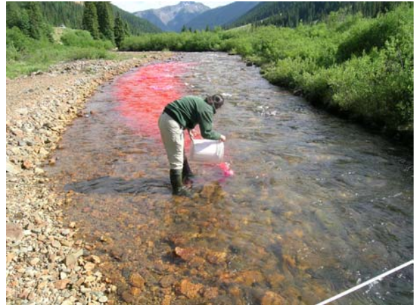
Degradable dye tracer is used to study stream - groundwater hydrology
