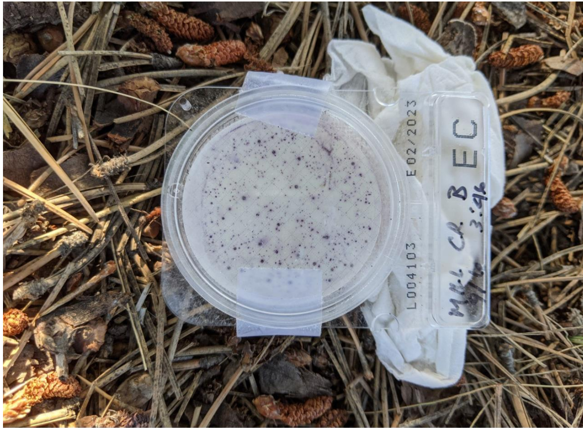
Figure 1: Agar plate used to grow E. Coli colonies in the field.
