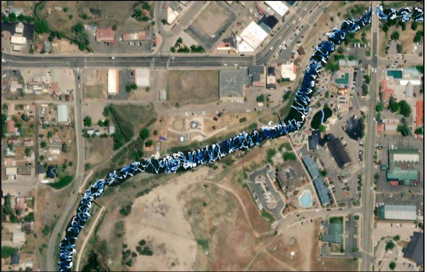
Figure 3. Bathymetric (underwater depth) survey data collected along the San Juan River in downtown Pagosa Springs. Data is being used to create hydraulic models of fish habitat quality and quantity.
